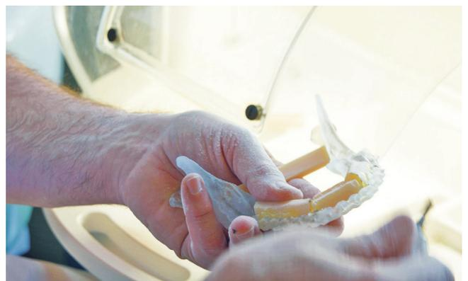
3D printed surgical guide produced on the Stratasys Objet260 Dental Selection 3D Printer.
