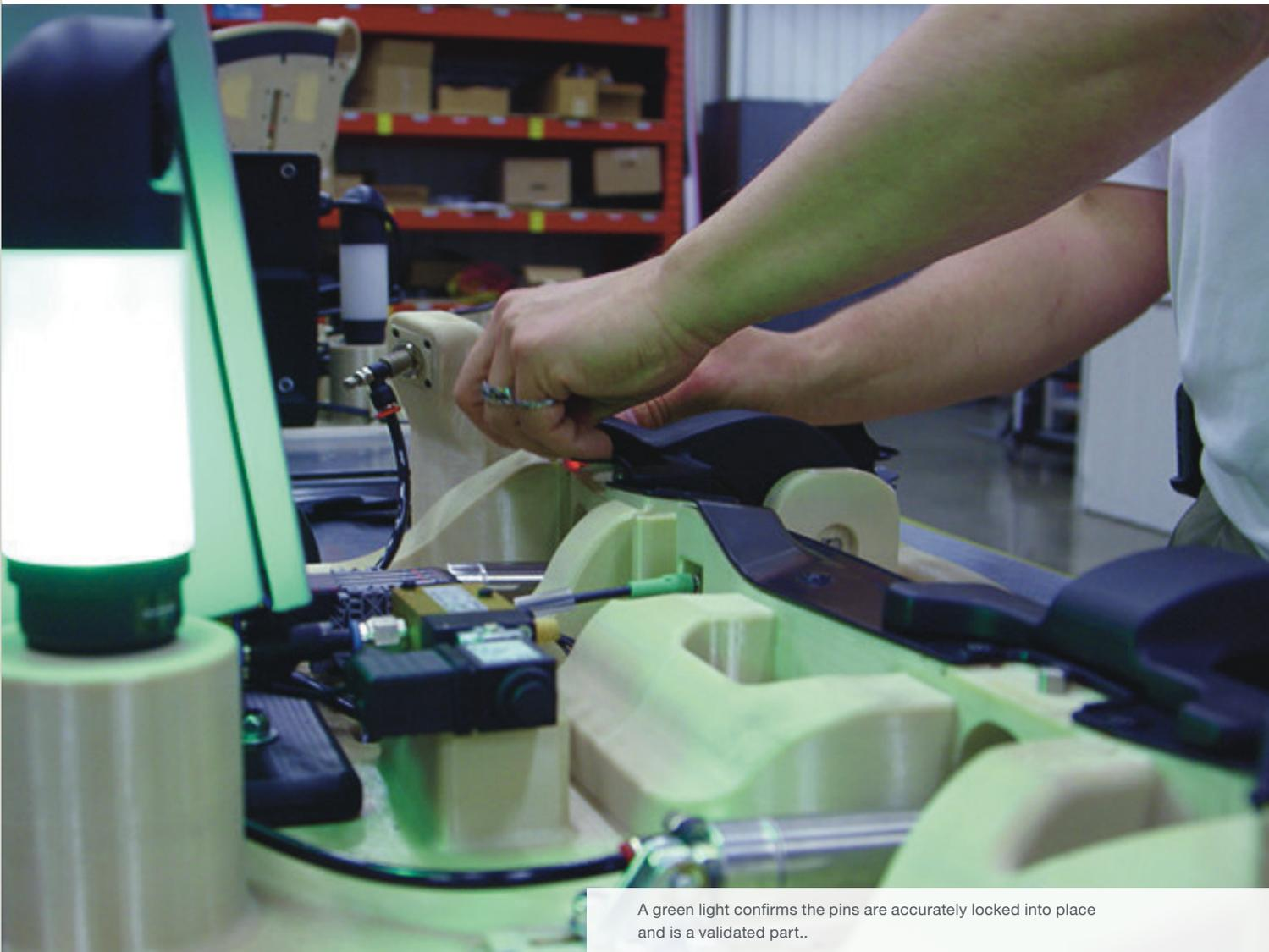
A green light confirms the pins are accurately locked into place and is a validated part..
