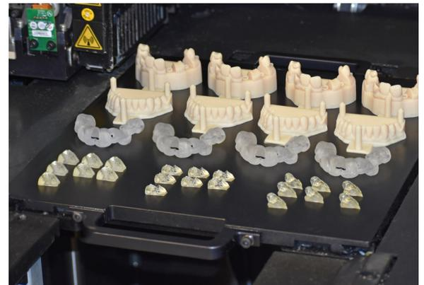
Arches printed in modeling material, guides in transparent, and gingival mask in flexible.
